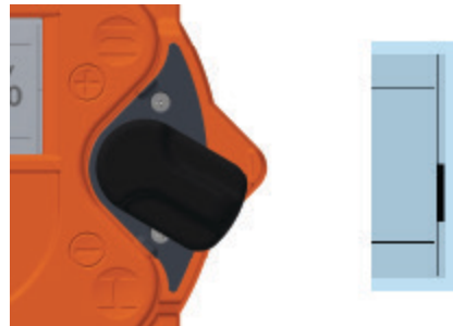
Figure 16 Control Switch End Limit Open
