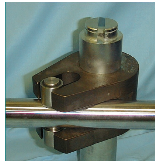
RGS F-Series yokes are dual arm, flat design to balance the forces and eliminate side loading of the shaft and bushings.
