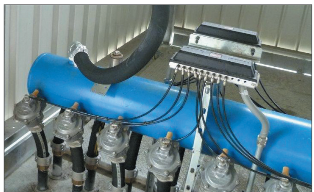
A two-stage pulse diaphragm valve. Threaded 2" connection with external control via pilot valve box.
