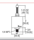
The SERIES 682 Industrial Pressure Transmitter is designed to withstand environmental effects such as shock, vibration, temperature, and EMI/RFI. The electronics and capacitive sensor are packaged in a welded stainless steel housing and meets NEMA 4 (IP65) protection ratings.
