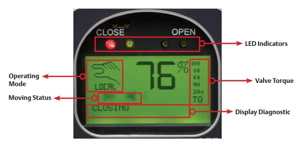
Once you follow the simple steps outlined in this guide, the actuator will be ready for normal operation. The bar graph, position digits, icons, and LEDs will indicate the valve status.
