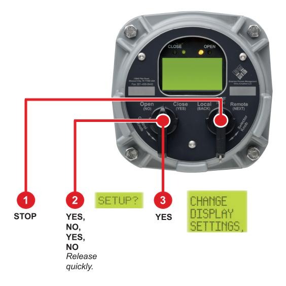
Turn the selector knob to the **STOP** position then toggle the control knob in rapid succession to **YES**, then **NO**, then **YES**, then **NO** and release. The setup icon will be displayed on the display module and "**SETUP?**" will be displayed on the message center. Rotate the control knob to **YES**. The message center will display "**CHANGE DISPLAY SETTINGS**".
