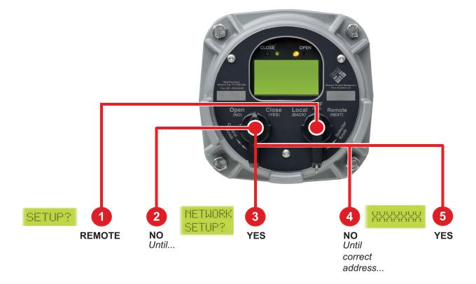
In the **"SETUP"** mode advance to **"NETWORK SETUP?"** using the selector knob in the **REMOTE** position. Answer **YES**. Hold the control knob in the NO position until the correct address appears. Answer **YES**. Unit is now network controlled. If other configuration changes are needed, please see the TEC2 Installation & Operation Manual (E2K-420-0117), which can be found at www.emerson/eim.
