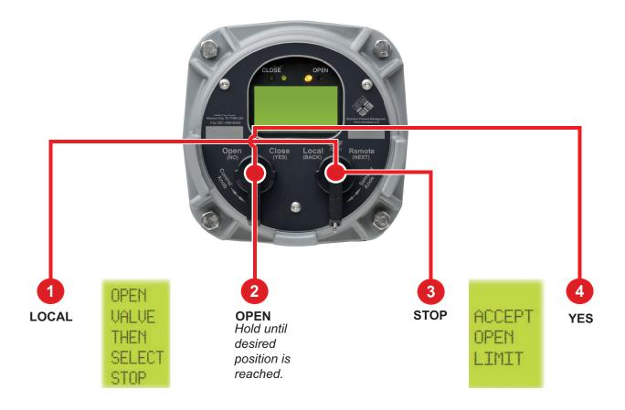
Turn the selector knob to the **"LOCAL"** position. Hold the control knob in the **"OPEN"** position until desired position is reached. Dis-engage motor drive by setting the declutch lever in **"HAND"** mode. Using handwheel, move the valve in the close direction for one handwheel turn to allow for motor coasting. Reengage motor drive by setting the declutch lever out of **"HAND"** mode.
