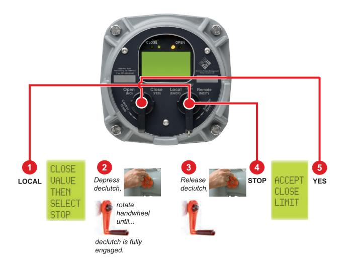
Turn the selector knob to the LOCAL position. At the "CLOSE VALVE THEN SELECT STOP" prompt, depress the declutch lever while rotating the handwheel until the clutch is fully engaged. Release the lever. When the valve is fully closed. Return the selector knob to the STOP position. At the "ACCEPT CLOSE LIMIT" prompt, select "YES."
