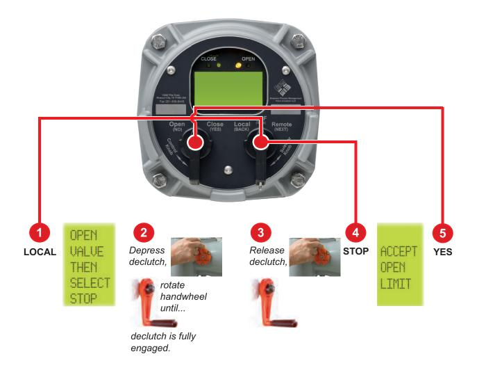
Turn the selector knob to the **LOCAL** position. At the **"OPEN VALVE THEN SELECT STOP"** prompt, depress the **declutch lever** while rotating the **handwheel** until the clutch is fully engaged. Release the lever. When the valve is fully opened. Return the selector knob to the **STOP** position. At the **"SAVE LIMITS"** prompt, select **"YES."**
