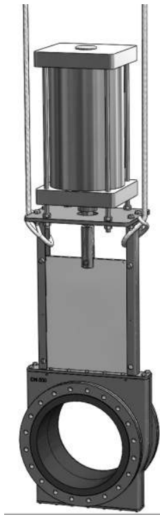
Figure 6. Valve lifting example.
