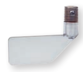
PDL-4 Minimum bulk density of 70 lb/ft 3 (1122 kg/m 3 ). Fits through 1-1/4" coupling eliminating the need for a mounting flange.
