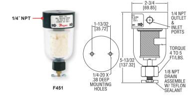
**MODEL F222 & F451** Compressed Air Filters protect equipment and instrumentation from harmful contaminant's such as dirt, water and oil. Liquids are continuously coalesced and released through the manual drain valves. Replaceable filter element removes particles and droplets as small as 0.01 micron with 93% efficiency. Units have 1/4" female NPT inlet and outlet and manual drain valve.
