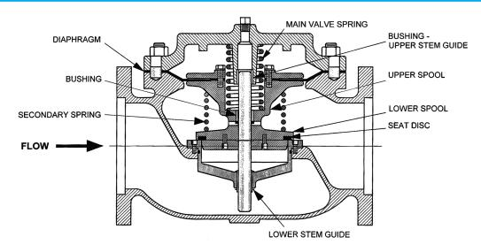
The 65SC/65SCA is full port valve equipped with a built in lift check feature to prevent backflow. When equipped with a variety of pilots and accessories the valve performs a wide range of automatic fluid control, while closing rapidly on reversal of pressure to prevent backflow.
