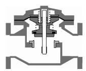
Valve inlet pressure is greater than valve outlet pressure. Pilot system controls valve to open.
