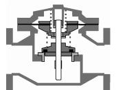
Valve inlet pressure is less than valve outlet pressure. The lift check (lower spool assembly) drops immediately to prevent reverse flow. The valve is closed and flow stops.
