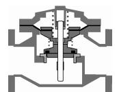
The upper spool assembly drops. The valve is now ready for normal forward flow operation.
