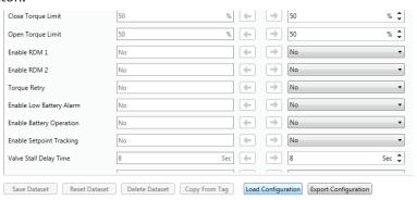
5. Load the configuration file from TEC2000 configuration file (\*.TEC or \*CFG)
