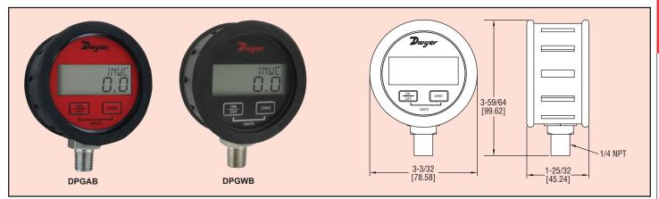
The Series <code>DPGWB/DPGAB</code> digital pressure gages offer 0.5% full-scale-accuracy in a rugged, easy-to-use unit at prices comparable to mechanical gauges. The DPGWB stainless steel wetted material makes it suitable for a wide variety of liquid or gases. The gages feature user-selectable units of measure allowing one gage to be used for a variety of pressure scales. The DPGWB/DPGAB come with a protective rubber boot to protect against short drops and rough handling.
