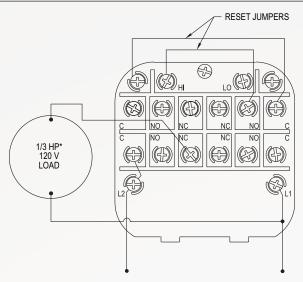
\*Note: For larger motors, use the Photohelic® Switch/Gage in a maintained contact, 120 Volt Control or Push Button Circuit of the motor starter.
