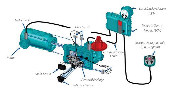
EIM Aquanaught actuators are a modular design – all critical components (motor, water sensor, limit and torque switches, hall effect sensor and electrical package) can be quickly disconnected for service at ease.
