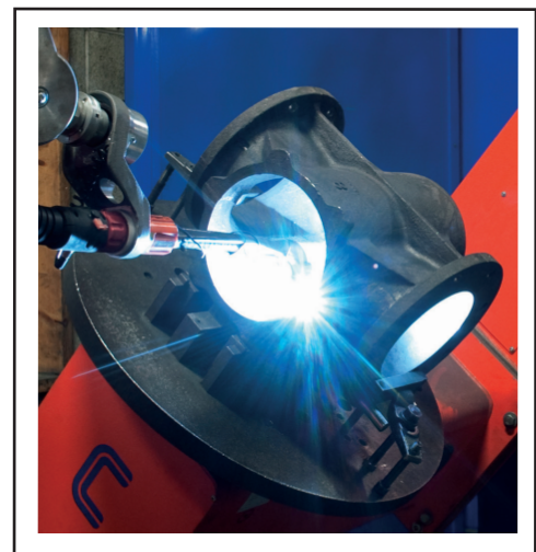
Figure 4. Robotic welding of nickel seat
