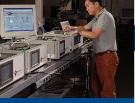
"Complete test lab with range of equipment allows EIM to load test any actuator at any electrical supply.
